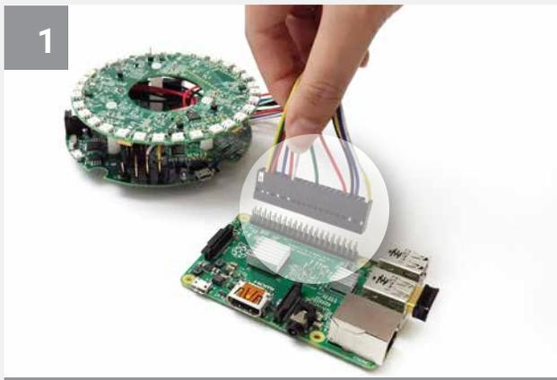
**1** Connect the cable assembly to the GPIO pins on the RPi 3. Align the sticker labeled '1' with physical pin 1 on the RPi 3.
