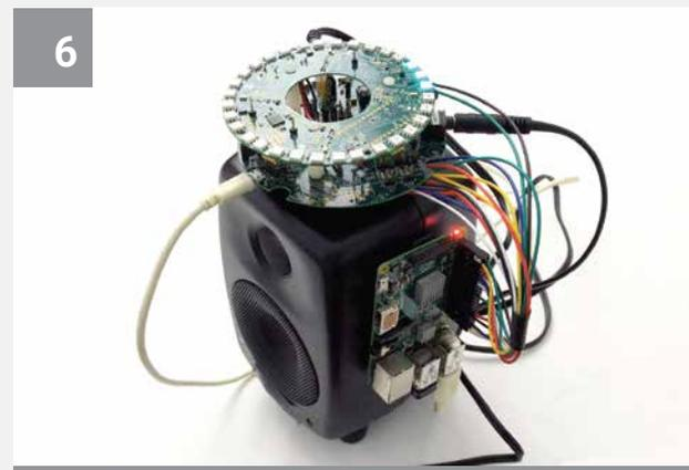
**6** The unit should be placed on top of the speaker and affixed with some putty or foam to minimize vibrations from the speaker.
