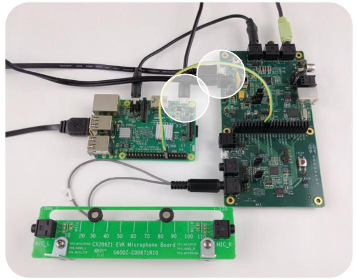
6 | Connect the power supplies for both CX20921 evaluation board, (J10, +5V power supply included) and RPi3 (J1). Switch the power switch (SW3) to turn on the CX20921 evaluation board. LED D6 (5V LED) will turn on when there is power on the board.
